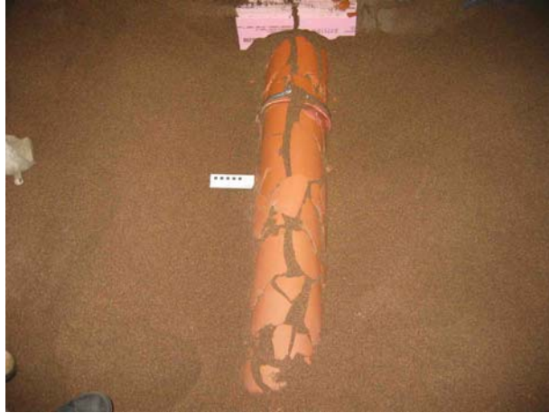
Figure 10. Photograph showing fractured clay pipe following excavation after the burst test.
