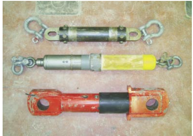
Fig. 1. Monitoring cells I, II, and III (top to bottom). Cell III is approximately 1 m long.
