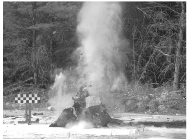
Fig. 1 – Blast-simulated rockburst event (136 milliseconds after detonation)
